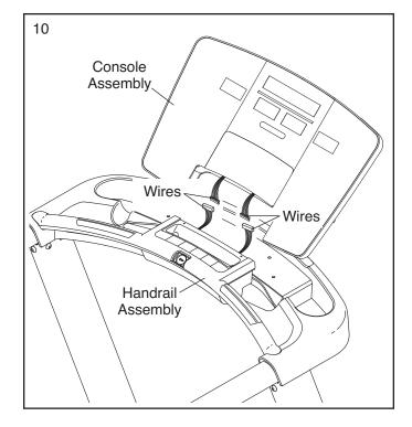
11. Insert the wires from the console assembly into the handrail assembly.
